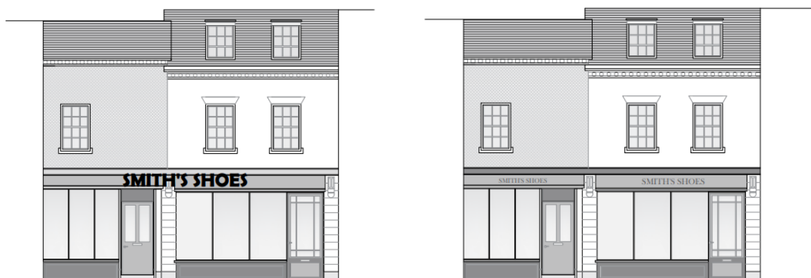
Graphic 1 Bad example (left) and good example (right) of signage on shopfront across more than one building
